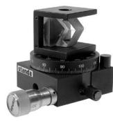
Closed type Fresnel Rhomb adapted for use with a Mini Rotation Stage 7R7.
