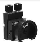
Connecting cone facilitates adjustment of the adapter to required position. The cut-off side clears the edge of the optics for working with a beam very closely situated to another beam. A fixing screw of stainless steel clutches optics firmly against two contact lines formed at the cut-off side.
