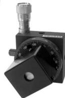
**Open type** Fresnel Rhomb adapted for use with a Mini Rotation Stage **7R7**.
