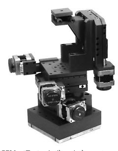
**50BM119T** – 2 axis tilt optical mount, three **8MT167-25** – motorized translation stages stacked in **XYZ** axes,
