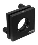
Beamsplitters/Optics Mount 5BM121 is designed for beamsplitters of Ø25.4 mm (1 inch). Fixing screw with a plastic tip clutches a beamsplitter against 2 contact lines. Mounting opening has a rest-flange designed to stop optics inside - its clear aperture is  $\emptyset$ **24 mm**.
