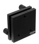
Universal Mirror Mount/Platform 5UM122 is suited for precise adjustments of standard mirrors which can be directly bound to it. The mount may also be used in horizontal position as a tilt table. Then it can be used to align opto-mechanics around two axes. For such mounting the Mount has an M4 hole on its back.
