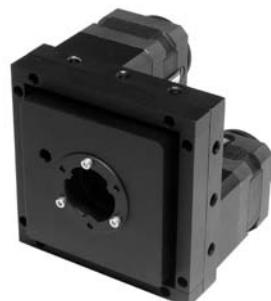
**Motorized Mirror Mounts 8MMA60** are designed for precise angular alignment of optical elements. Platform is **tilted about two axes**. A **retaining ring** keeps optics in a non-through mounting opening of the platform.
