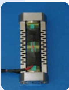
Figure 4.16: View of the PPA40L Actuator
