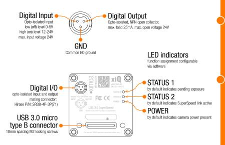
Digital I/O pinout (rear panel view)
